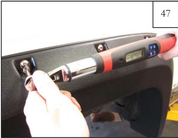
With the edge trim in place and once all screws have been started, snug screws to vehicle. Torque screws to 24 in•lb (2 ft•lb). DO NOT OVERTIGHTEN!
