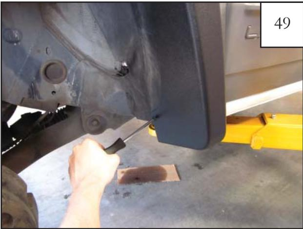
Using a philips screwdriver, install supplied screw (SW1-0056) into hole drilled in step 47.
